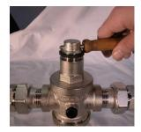
All pressure reducers are tested before being packaged; during the proof they are pre-set at the outlet pressure of 3 bars; outlet pressure can be easely adjusted once the pressure reducing valve in installed on site.
